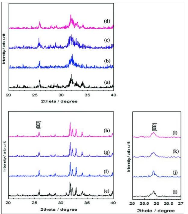
The pure HA phase can be obtained by heating the as-prepared powder at 1000 °C with the stirring speed above 400 rpm as shown on Fig. 1f–h. The FWHM at (002) peak is widen with the increasing of stirring speed as shown on Fig. 1i–l leading to reduce the CS calculated by Scherer equation. The effect of RN on CS is shown on Fig. 2.
