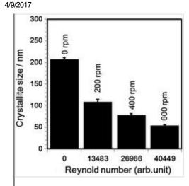
B. Effect of stirring mode on the CS of HA synthesized calculated from SEM
